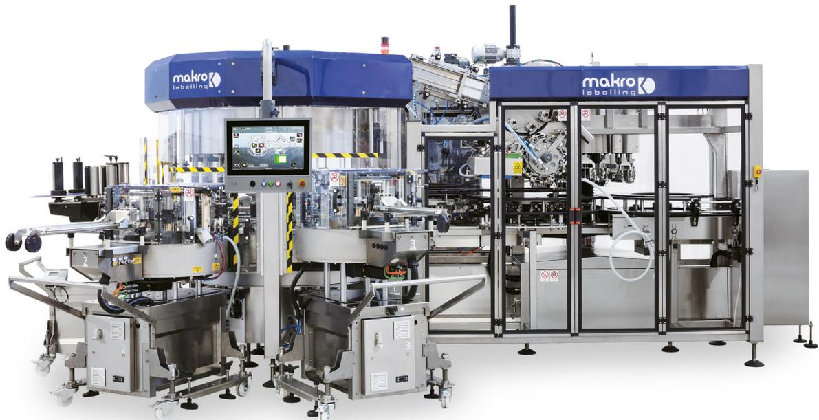
**5, 6, 7 and 8** labellers, on the other hand, satisfy the needs of medium to large companies. The range includes a high speed self-adhesive labeller with reel winders and non-stop system enabling production to continue at maximum speed even during reel changes and a combined labeller to apply the fiscal guarantee seal.
